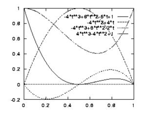
The curves for  $\underline{y}(t)$  and z(t) are <u>contructed</u> in an analogous fashion to that for x(t). The basis matrix and basis functions thus remain the same. Only the geometry vector changes. The geometry vector for  $\underline{y}(t)$  gives the y components of P0, P0.5, T0.5, and P1. In general, we can write the curve as a single vector equation
