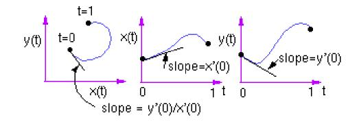
Suppose we wish to define a cubic curve such that the user specifies the position of two endpoints and a midpoint, as well as the tangent at the midpoint. The following figure illustrates some sample curves.
